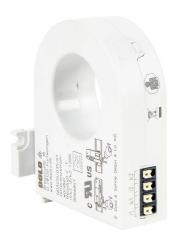
Dold AC/DC current transformer, solid core, 35mm diameter sensing window, +/- 3% accuracy. For use with Dold RN5883-001-24-80V or RN5883-001-80-230V residual current monitors.
