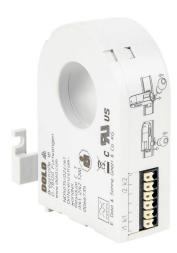
Dold AC/DC current transformer, solid core, 24mm diameter sensing window, +/- 3% accuracy. For use with Dold RN5883-001-24-80V or RN5883-001-80-230V residual current monitors.
