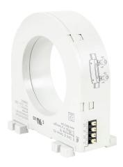
Dold AC/DC current transformer, solid core, 70mm diameter sensing window, +/- 3% accuracy. For use with Dold RN5883-011-24-80V or RN5883-011-80-230V residual current monitors.
