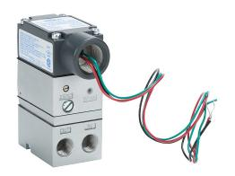
NITRA compact current to pneumatic transducer, 4-20 mA input, 6 to 30 psig output pressure, 1/4in female NPT inlet(s), 1/4in female NPT outlet(s), 1/2in female NPT with 12in wire leads, NEMA 4X, IP65. Mounting bracket included.
