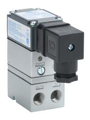
NITRA compact current to pneumatic transducer, 4-20 mA input, 6 to 30 psig output pressure, 1/4in female NPT inlet(s), 1/4in female NPT outlet(s), DIN 43650 connector, NEMA 4X, IP65. Mounting bracket included.
