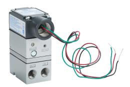
NITRA compact current to pneumatic transducer, 4-20 mA input, 3 to 27 psig output pressure, 1/4in female NPT inlet(s), 1/4in female NPT outlet(s), 1/2in female NPT with 12in wire leads, NEMA 4X, IP65. Mounting bracket included.
