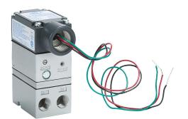
NITRA compact current to pneumatic transducer, 4-20 mA input, 3 to 27 psig output pressure, 1/4in female NPT inlet(s), 1/4in female NPT outlet(s), 1/2in female NPT with 12in wire leads, NEMA 4X, IP65. Mounting bracket included.
