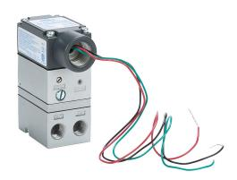
NITRA compact current to pneumatic transducer, 4-20 mA input, 3 to 15 psig output pressure, 1/4in female NPT inlet(s), 1/4in female NPT outlet(s), 1/2in female NPT with 12in wire leads, NEMA 4X, IP65. Mounting bracket included.
