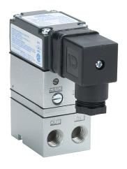
NITRA compact current to pneumatic transducer, 4-20 mA input, 3 to 15 psig output pressure, 1/4in female NPT inlet(s), 1/4in female NPT outlet(s), DIN 43650 connector, NEMA 4X, IP65. Mounting bracket included.
