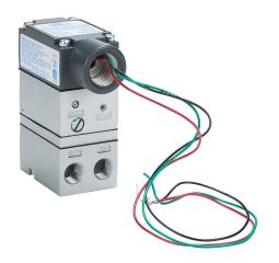
NITRA compact current to pneumatic transducer, 4-20 mA input, 3 to 120 psig output pressure, 1/4in female NPT inlet(s), 1/4in female NPT outlet(s), 1/2in female NPT with 12in wire leads, NEMA 4X, IP65. Mounting bracket included.
