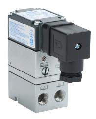
NITRA compact current to pneumatic transducer, 4-20 mA input, 3 to 120 psig output pressure, 1/4in female NPT inlet(s), 1/4in female NPT outlet(s), DIN 43650 connector, NEMA 4X, IP65. Mounting bracket included.
