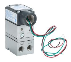
NITRA compact current to pneumatic transducer, 4-20 mA input, 2 to 60 psig output pressure, 1/4in female NPT inlet(s), 1/4in female NPT outlet(s), 1/2in female NPT with 12in wire leads, NEMA 4X, IP65. Mounting bracket included.
