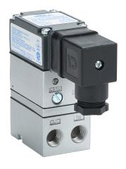
NITRA compact current to pneumatic transducer, 4-20 mA input, 2 to 60 psig output pressure, 1/4in female NPT inlet(s), 1/4in female NPT outlet(s), DIN 43650 connector, NEMA 4X, IP65. Mounting bracket included.
