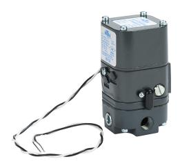
NITRA current to pneumatic transducer, 4-20 mA input, 6 to 30 psig output pressure, 1/4in female NPT inlet(s), 1/4in female NPT outlet(s), 1/2in female NPT with 12in wire leads, NEMA 4X, IP65. Mounting bracket included.
