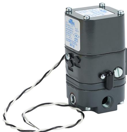
NITRA current to pneumatic transducer, 4-20 mA input, 3 to 27 psig output pressure, 1/4in female NPT inlet(s), 1/4in female NPT outlet(s), 1/2in female NPT with 12in wire leads, NEMA 4X, IP65. Mounting bracket included.
