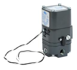
NITRA current to pneumatic transducer, 4-20 mA input, 3 to 15 psig output pressure, 1/4in female NPT inlet(s), 1/4in female NPT outlet(s), 1/2in female NPT with 12in wire leads, NEMA 4X, IP65. Mounting bracket included.
