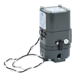
NITRA current to pneumatic transducer, 4-20 mA input, 3 to 120 psig output pressure, 1/4in female NPT inlet(s), 1/4in female NPT outlet(s), 1/2in female NPT with 12in wire leads, NEMA 4X, IP65. Mounting bracket included.
