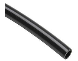
NITRA pneumatic tubing, nylon 12, black, 5/16in (8mm) outside diameter, 6mm inside diameter, 500ft reel.
