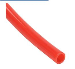
NITRA pneumatic tubing, nylon 12, red, 6mm outside diameter, 5/32in (4mm) inside diameter, 500ft reel.
