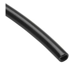
NITRA pneumatic tubing, nylon 12, black, 6mm outside diameter, 5/32in (4mm) inside diameter, 500ft reel.
