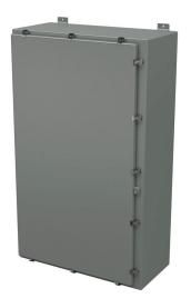
Stahlin N series enclosure, NEMA 1/3/3R/4X/12, 60 x 36 x 16in (HxWxD), wall mount, fiberglass reinforced polyester, gray, single-door, (11) twist-lock latches, padlock hasp and staple.
