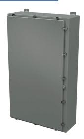
Stahlin N series enclosure, NEMA 1/3/3R/4X/12, 60 x 36 x 12in (HxWxD), wall mount, fiberglass reinforced polyester, gray, single-door, (11) twist-lock latches, padlock hasp and staple.
