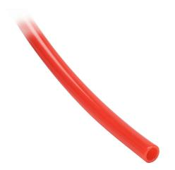
NITRA pneumatic tubing, nylon 12, red, 5/32in (4mm) outside diameter, 0.106in inside diameter, 500ft reel.
