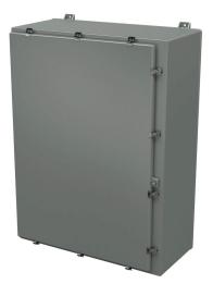
Stahlin N series enclosure, NEMA 1/3/3R/4X/12, 48 x 36 x 16in (HxWxD), wall mount, fiberglass reinforced polyester, gray, single-door, (10) twist-lock latches, padlock hasp and staple.
