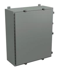
Wiegmann enclosure, NEMA 4/12/13, 36 x 30 x 12in (HxWxD), wall mount, carbon steel, ANSI 61 gray, powder coat finish, single-door, (7) stainless steel clamps, padlock hasp and staple.
