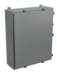
Wiegmann enclosure, NEMA 4/12/13, 36 x 30 x 10in (HxWxD), wall mount, carbon steel, ANSI 61 gray, powder coat finish, single-door, (7) stainless steel clamps, padlock hasp and staple.
