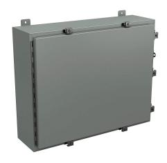
Wiegmann enclosure, NEMA 4/12/13, 24 x 30 x 8in (HxWxD), wall mount, carbon steel, ANSI 61 gray, powder coat finish, single-door, (7) stainless steel clamps, padlock hasp and staple.
