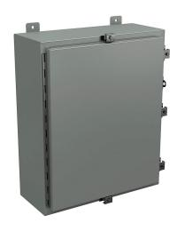
Wiegmann enclosure, NEMA 4/12/13, 24 x 20 x 8in (HxWxD), wall mount, carbon steel, ANSI 61 gray, powder coat finish, singledoor, (5) stainless steel clamps, padlock hasp and staple.
