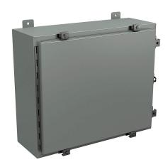
Wiegmann enclosure, NEMA 4/12/13, 20 x 24 x 8in (HxWxD), wall mount, carbon steel, ANSI 61 gray, powder coat finish, singledoor, (6) stainless steel clamps, padlock hasp and staple.
