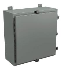
Wiegmann enclosure, NEMA 4/12/13, 20 x 20 x 8in (HxWxD), wall mount, carbon steel, ANSI 61 gray, powder coat finish, single-door, (4) stainless steel clamps, padlock hasp and staple.
