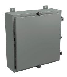
Wiegmann enclosure, NEMA 4/12/13, 20 x 20 x 6in (HxWxD), wall mount, carbon steel, ANSI 61 gray, powder coat finish, singledoor, (4) stainless steel clamps, padlock hasp and staple.
