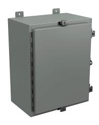
Wiegmann enclosure, NEMA 4/12/13, 20 x 16 x 10in (HxWxD), wall mount, carbon steel, ANSI 61 gray, powder coat finish, single-door, (4) stainless steel clamps, padlock hasp and staple.
