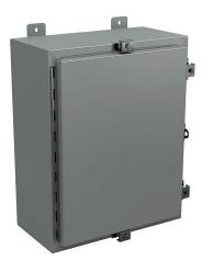
Wiegmann enclosure, NEMA 4/12/13, 20 x 16 x 8in (HxWxD), wall mount, carbon steel, ANSI 61 gray, powder coat finish, single-door, (4) stainless steel clamps, padlock hasp and staple.
