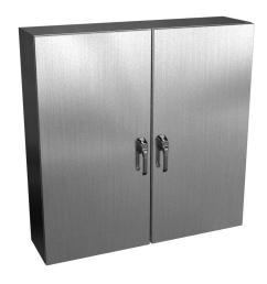
Wiegmann Ultimate series enclosure, NEMA 3R/4/4X/12/13, 48 x 48 x 12in (HxWxD), wall mount, 304 stainless steel, No. 3 intermediate polished finish, 2-door, 3-point keylocking/padlocking combo handle.
