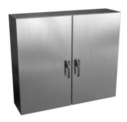
Wiegmann Ultimate series enclosure, NEMA 3R/4/4X/12/13, 42 x 48 x 12in (HxWxD), wall mount, 304 stainless steel, No. 3 intermediate polished finish, 2-door, 3-point keylocking/padlocking combo handle.
