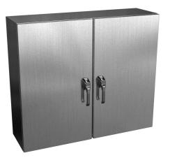
Wiegmann Ultimate series enclosure, NEMA 3R/4/4X/12/13, 36 x 42 x 12in (HxWxD), wall mount, 304 stainless steel, No. 3 intermediate polished finish, 2-door, 3-point keylocking/ padlocking combo handle.
