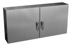
Wiegmann Ultimate series enclosure, NEMA 3R/4/4X/12/13, 30 x 60 x 10in (HxWxD), wall mount, 304 stainless steel, No. 3 intermediate polished finish, 2-door, 3-point keylocking/ padlocking combo handle.
