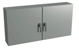
Wiegmann Ultimate series enclosure, NEMA 3R/4/12/13, 30 x 60 x 10in (HxWxD), wall mount, carbon steel, ANSI 61 gray, powder coat finish, 2-door, 3-point keylocking/padlocking combo handle.
