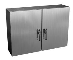
Wiegmann Ultimate series enclosure, NEMA 3R/4/4X/12/13,  $30 \times 42 \times 10$  in (HxWxD), wall mount, 304 stainless steel, No. 3 intermediate polished finish, 2-door, 3-point keylocking/padlocking combo handle.
