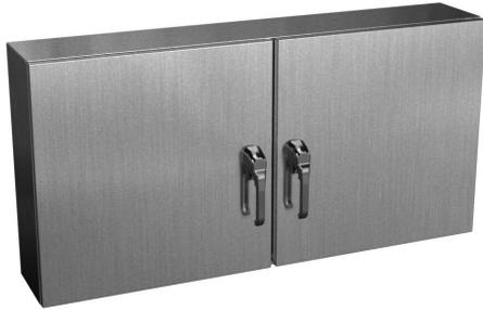
Wiegmann Ultimate series enclosure, NEMA 3R/4/4X/12/13, 24 x 48 x 8in (HxWxD), wall mount, 304 stainless steel, No. 3 intermediate polished finish, 2-door, 3-point keylocking/padlocking combo handle.
