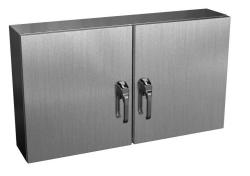
Wiegmann Ultimate series enclosure, NEMA 3R/4/4X/12/13, 24 x 42 x 8in (HxWxD), wall mount, 304 stainless steel, No. 3 intermediate polished finish, 2-door, 3-point keylocking/ padlocking combo handle.
