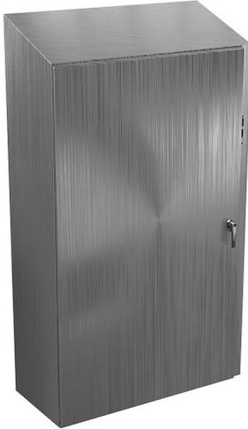
Wiegmann Ultimate series disconnect enclosure, slope top, NEMA 4/4X/12/13, right flange, 60 x 38 x 16in (HxWxD), wall mount, 304 stainless steel, No. 3 intermediate polished finish, single-door, 3-point padlocking handle, purchase subpanel separately.
