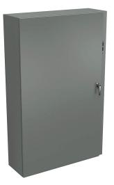
Wiegmann Ultimate series disconnect enclosure, NEMA 4/12/13, right flange, 60 x 38 x 12in (HxWxD), wall mount, carbon steel, ANSI 61 gray, powder coat finish, single-door, 3-point padlocking handle, purchase subpanel separately.
