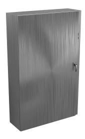
Wiegmann Ultimate series disconnect enclosure, NEMA 4/4X/12/13, right flange, 60 x 38 x 12in (HxWxD), wall mount, 316L stainless steel, No. 3 intermediate polished finish, single-door, 3-point padlocking handle, purchase subpanel separately.
