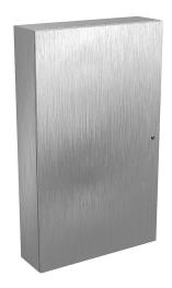
Wiegmann Ultimate series enclosure, NEMA 4/4X/12/13, 60 x 36 x 10in (HxWxD), wall mount, 304 stainless steel, No. 3 intermediate polished finish, single-door, 1/4-turn semi-flush oil-tight latch.
