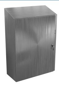
Wiegmann Ultimate series disconnect enclosure, slope top, NEMA 4/4X/12/13, right flange, 48 x 38 x 16in (HxWxD), wall mount, 304 stainless steel, No. 3 intermediate polished finish, singledoor, 3-point padlocking handle, purchase subpanel separately.
