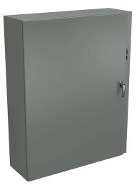
Wiegmann Ultimate series disconnect enclosure, NEMA 4/12/13, right flange, 48 x 38 x 12in (HxWxD), wall mount, carbon steel, ANSI 61 gray, powder coat finish, single-door, 3-point padlocking handle, purchase subpanel separately.
