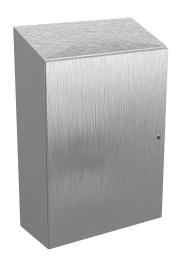
Wiegmann Ultimate series enclosure, slope top, NEMA 4/4X/12/13,  $48 \times 36 \times 16$  in (HxWxD), wall mount, 304 stainless steel, No. 3 intermediate polished finish, single-door, 1/4-turn semi-flush oil-tight latch.
