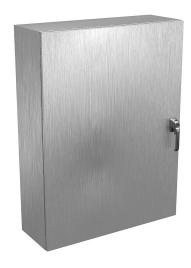
Wiegmann Ultimate series enclosure, NEMA 4X/12/13,  $48 \times 36 \times 12$  in (HxWxD), wall mount, 304 stainless steel, No. 3 intermediate polished finish, single-door, 3-point 316L padlocking handle.
