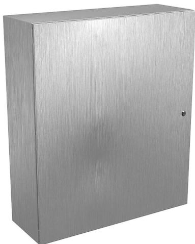
Wiegmann Ultimate series enclosure, NEMA 4/4X/12/13, 42 x 36 x 12in (HxWxD), wall mount, 304 stainless steel, No. 3 intermediate polished finish, single-door, 1/4-turn semi-flush oil-tight latch.
