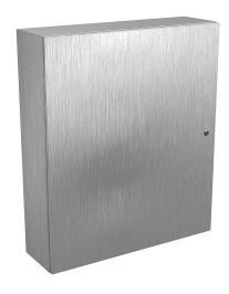
Wiegmann Ultimate series enclosure, NEMA 4/4X/12/13,  $42 \times 36 \times 10$  in (HxWxD), wall mount, 304 stainless steel, No. 3 intermediate polished finish, single-door, 1/4-turn semi-flush oil-tight latch.
